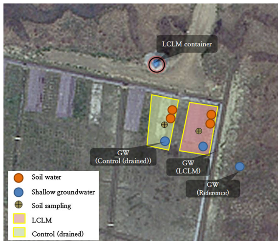
(a) Monitoring points with drainage system
